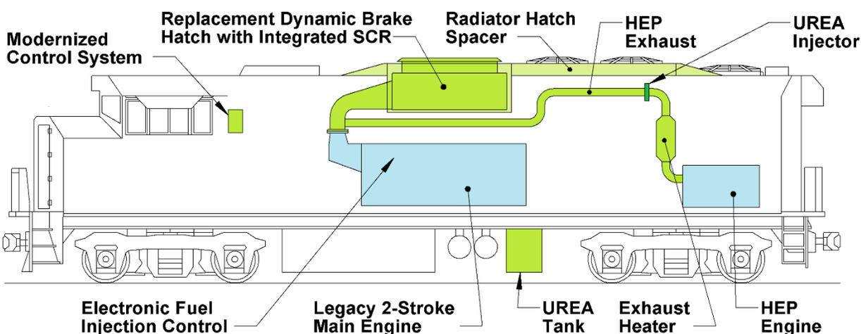
DEF flow to the exhaust is controlled by a programmable logic controller (PLC) driving a variable-speed volumetric metering pump. The flow rate is calculated from the estimated exhaust NO<sub>x</sub> flow rate, based on the measured power outputs of the main and HEP engines.
